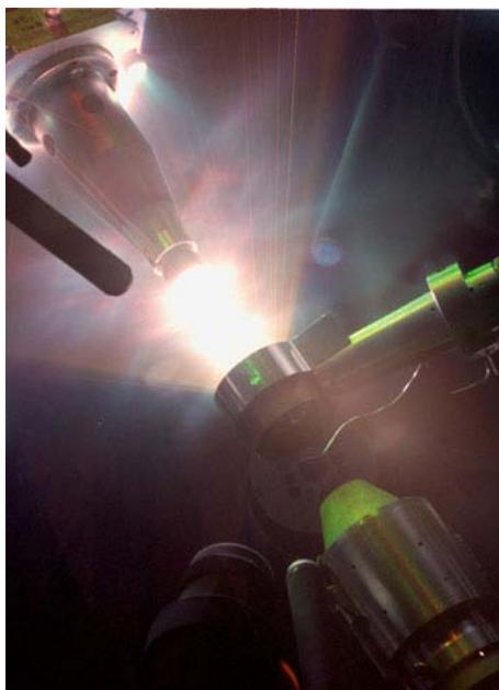
Fig. 3.8 Laser-driven shock-wave compression of a substance precompressed in a diamond anvil at the OMEGA facility [69].
